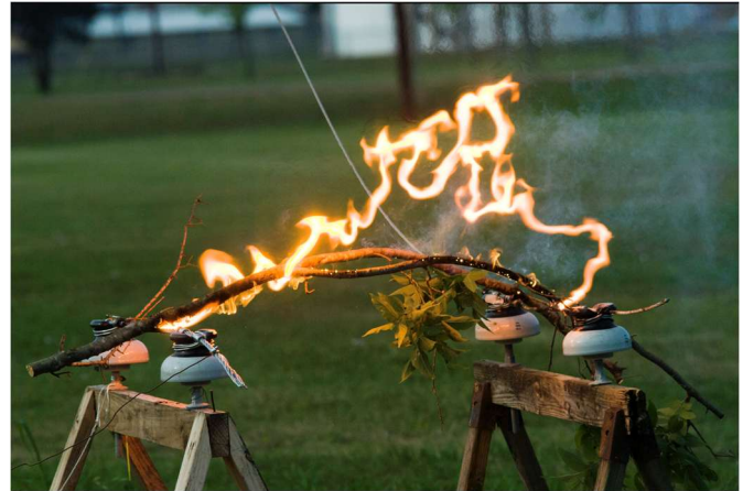
Fig. 2: Flashover produced by vegetation contact.
