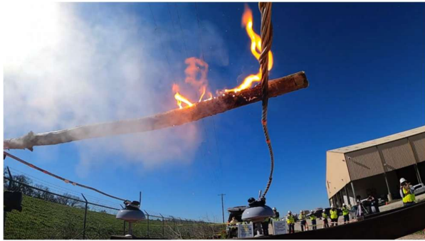
Figure 4: Arcing visible at sub-ampere current levels
