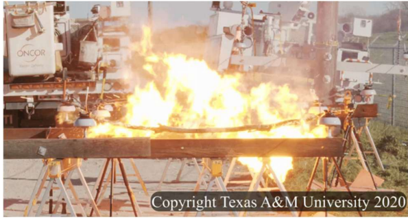
Figure 3: Extinguishing of high-current arc from 2020 tests.
