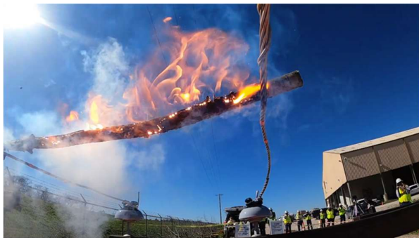
Figure 5: Flames and arcing just before flashover
